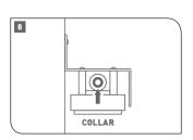
**NOTE**: Routine maintenance and cartridge replacement will not require that you disconnect the tubing from the system head; however, tubing may be quickly and easily removed from the fitting if necessary. First, turn off the water supply to the filter. Open kitchen faucet, then press in the collar around the fitting while pulling the tubing with your hand.
